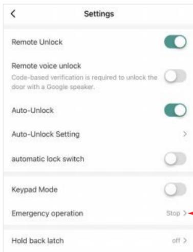
The emergency operation is intended to provide a control operation that can be rotated in a specified direction when the Smart Lock is in an abnormal state.
